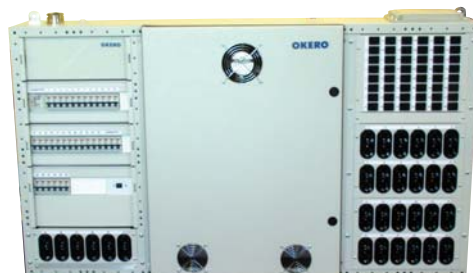
24*13A OKERO SID cabinet equipped with power patching consisting of 24 dimmed and 6 non-dimmed twin Schuko outlets and 48 inputs connected to terminals. This dimmer is also equipped with an 80A mains breaker.
